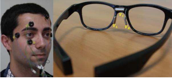
Fig. 4. (a) Conventional, gel-based electrode configuration, (b) JINS MEME electrode configuration
